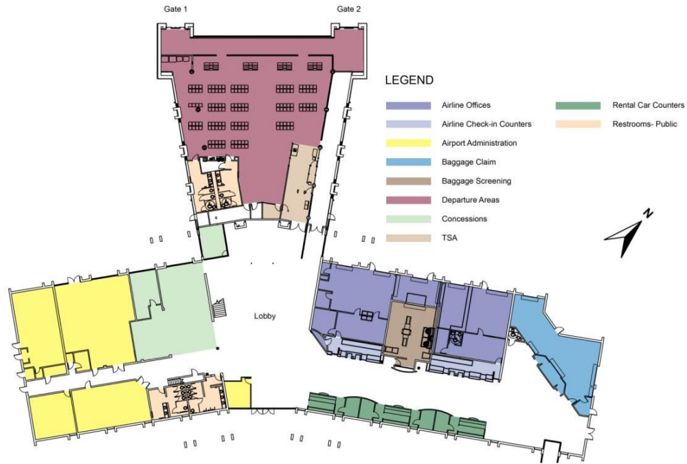
Figure 3-4 PASSENGER TERMINAL FLOOR PLANS
